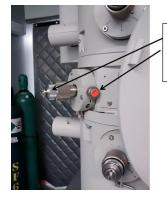
This is a side view of the objective aperture, but adjustments to condensor aperture 2 is the same
